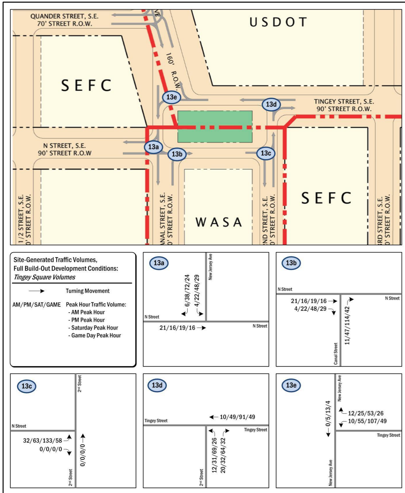
Figure 38: Tingley Square Site-Generated Peak Hour Traffic Volumes for Full Build-Out
